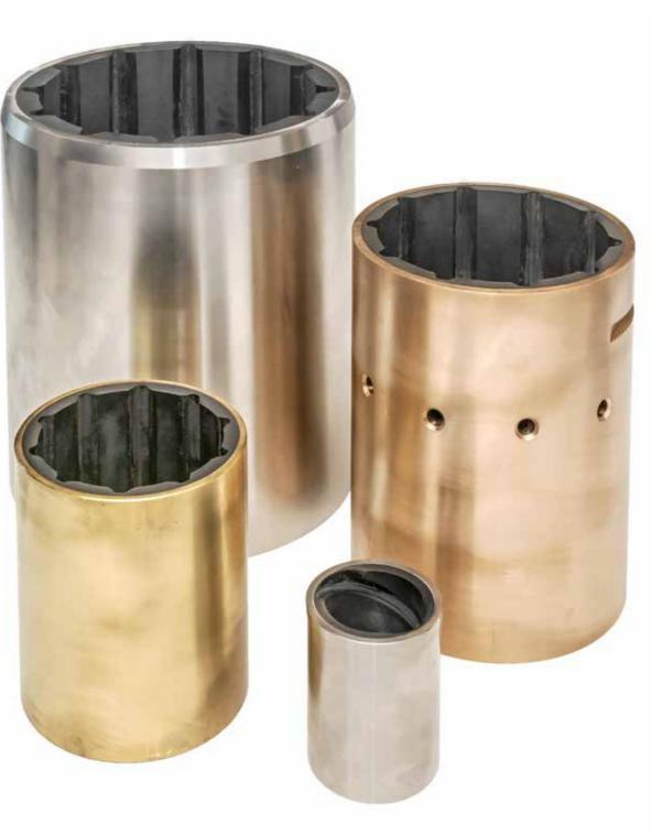
The flexibility of the bearing surface allows adjustment of the approach angle in response to an applied load to maintain water-wedges, acting in a similar manner to modern tilting pad thrust bearings to maintain the film thickness.
